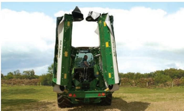
For transportation, the McHale Pro Glide folds vertically to position itself behind the centre point of the tractor for safe transport.
