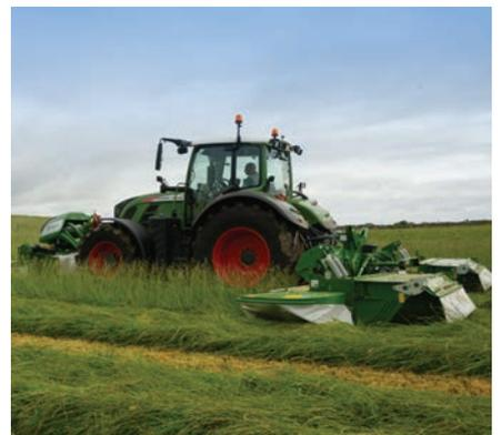
The Pro Glide range of rear mowers are fitted with patented ground adaption technology, which allows the bed to move back and up if the bed encounters small obstacles. This saves time and maximises throughput as it means the obstacle does not trigger the main break back protection. This results in higher moving speeds being able to be achieved without the interruption of having to reset the break back.
