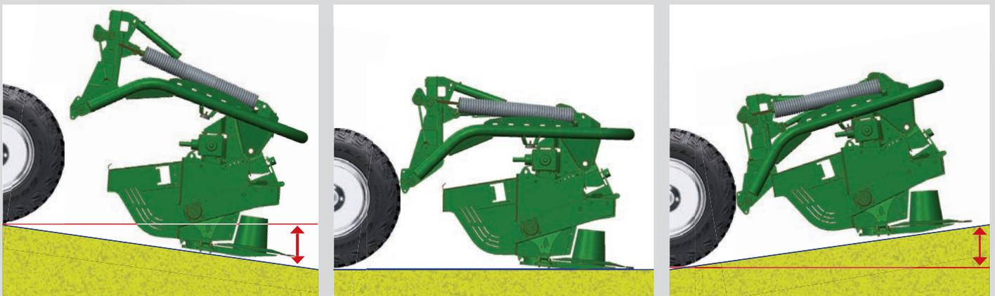
The ProGlide front mower has its own independent suspension, which allows the mower to automatically move up & down independent of the tractor and has a vertical travel range of 500 mm. If mowing into a dip the angle of the cutterbar will automatically adjust down and while mowing into an incline the cutterbar angle will automatically adjust up.
