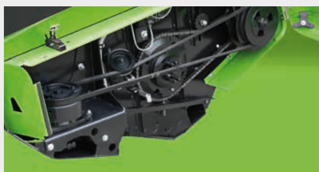
↑ Epicyclic gearing with 1,220 cuts/min for a high cutting frequency.
