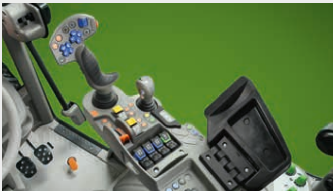
↑ The MaxCom armrest with ergonomic joystick and clearly colour coded functions.
