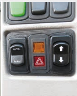
↑ Independent control between front BALANCE and rear levelling system, both with automatic or manual function.
