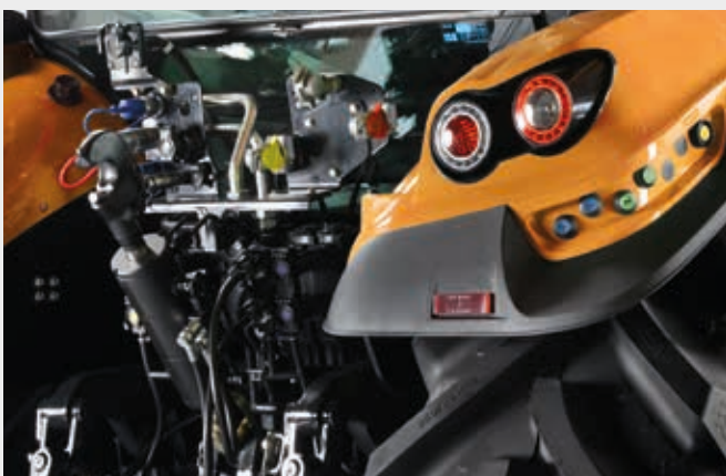
The pneumatic trailer brake system decelerates trailers in all weight categories reliable and safely.
