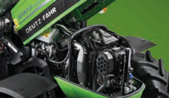
↑ Compact radiator with Visco fan and PowerCore air filter for maximum engine efficiency.
