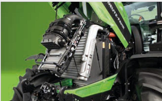
Aluminium cooling system of 6210 TTV, 6230 TTV and 6230 TTV HD with one-hand access lever and Powercore air filter.
