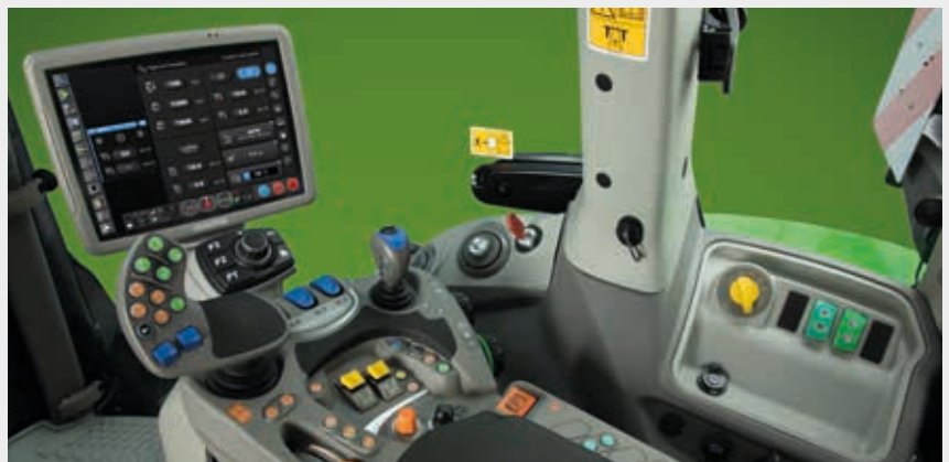
↑ The MaxCom armrest of the 7 Series TTV incorporates all the main controls and allows total management of the machine.
