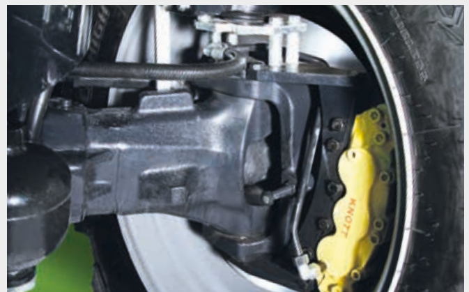
↑ 60 kph and maximum braking power with external dry disc brakes.
