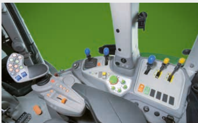
RCshift transmission: MaxCom Joystick always included.
