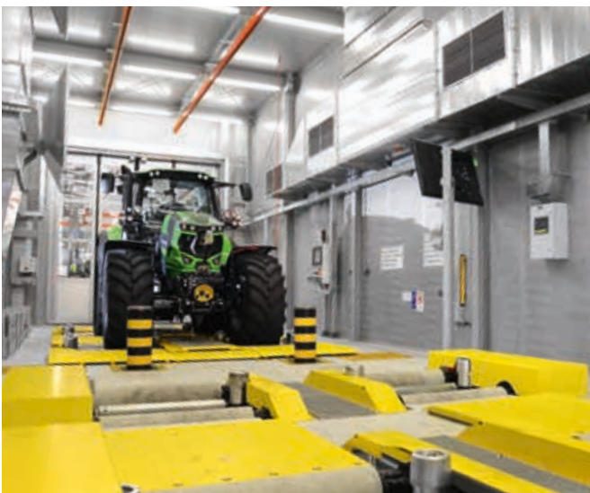
↑ Lauingen, Germany: unique in tractor production: the axle and chassis dynamometers.
