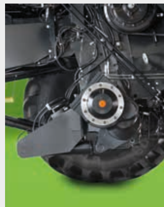
↑ The 25 t capacity axles allow the machine to work in the most extreme conditions, ensuring utmost reliability and, above all, driver safety.
