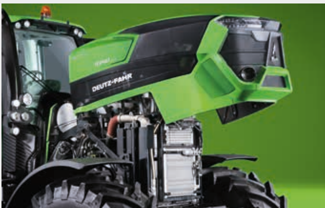
↑ An electrically opening hood facilitates maintenance work.
