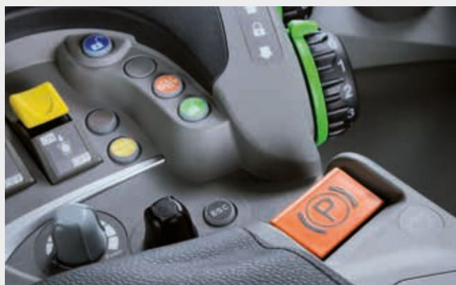
↑ Electronic Parking Brake (EPB) integrated into MaxCom armrest.
