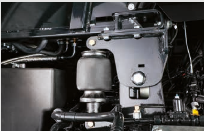
↑ The 8280 TTV can be equipped with pneumatic cab suspension.
