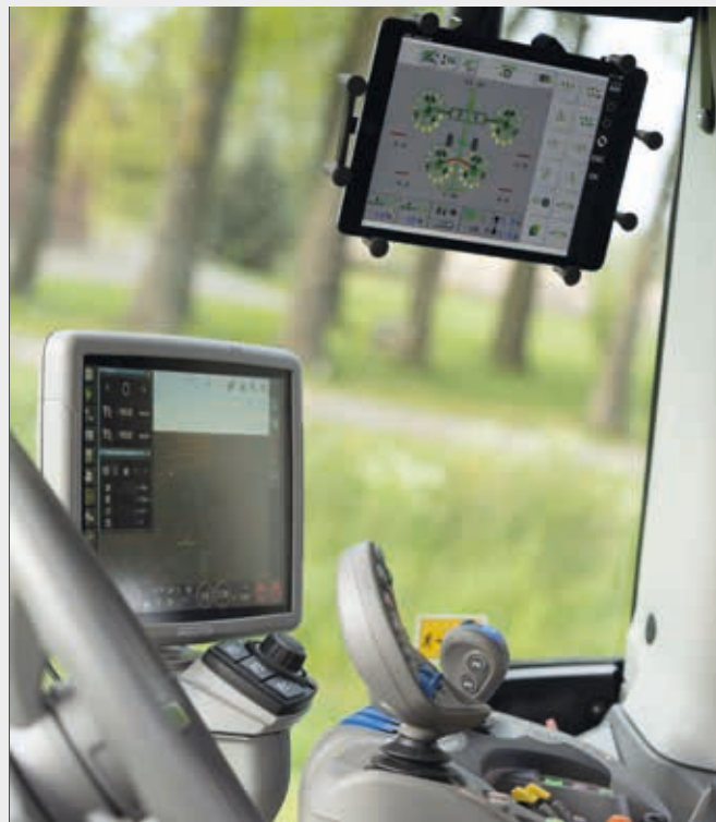
↑ The XTEND function allows the display of SDF Guidance or let you control an ISOBUS implement on an external device, e.g. a tablet.
