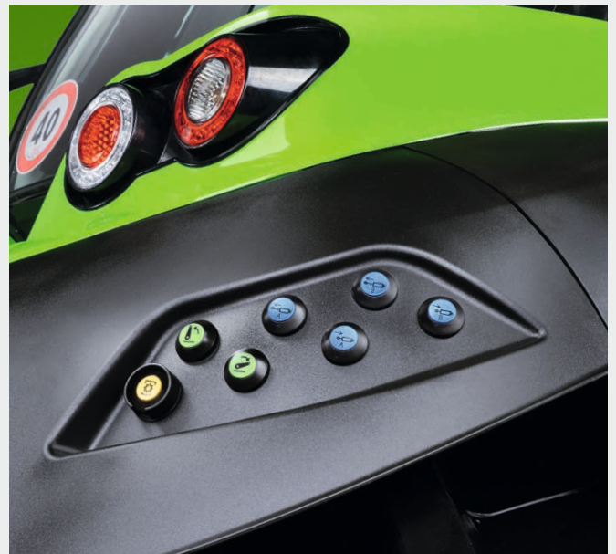
↑ External control of the hydraulics and PTO functions from either side.
