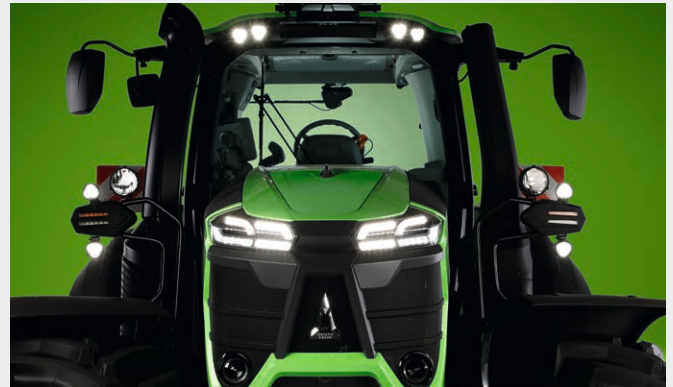
↑ LED package with up to 40,000 lm.
