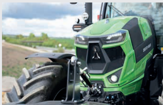
↑ LED driving lights and characteristic LED worklights.
