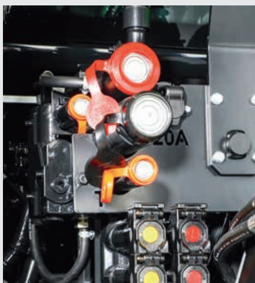
⬆ Power Beyond with flat face couplers for a clean connection.
