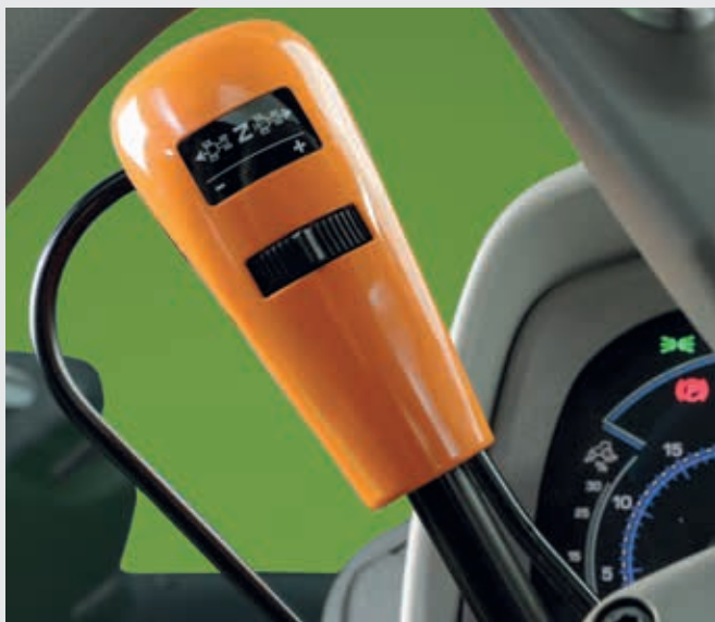
↑ PowerShuttle with Sense Clutch and five direction change settings.
